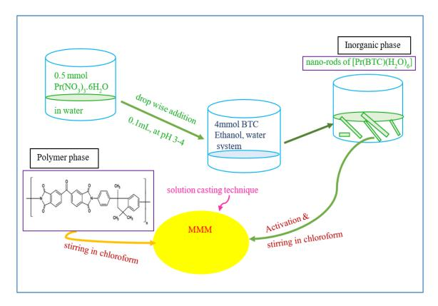
Fig. 1: Graphical abstract representing formation of MOF and fabrication of  $[Pr(BTC)(H_2O)_6]$ -Matrimid MMMs through incorporation of inorganic  $[Pr(BTC)(H_2O)_6]$  filler.
