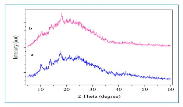
Fig. 5: Powder XRD patterns of MMMs with 10 wt.% a and b 30 wt. % MOF.
