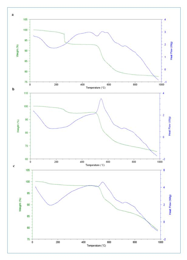
Fig. 6: Thermograms and DSC for 10~a~20~b and 30~c~wt.% MMM.
