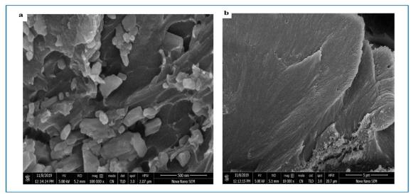
Fig. 7: SEM micrographs of MMM with 10 wt.% loading at 500 nm a and 5 μm b resolution
