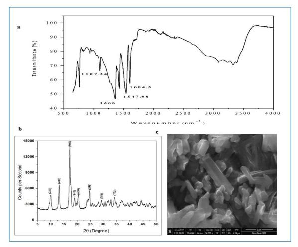
Fig. 3: FTIR spectrum **a** simulated powder XRD pattern **b** scanning electron micrograph at 1 $\mu$ m resolution **c** for [Pr(BTC)(H<sub>2</sub>O)<sub>6</sub>] MOF.
