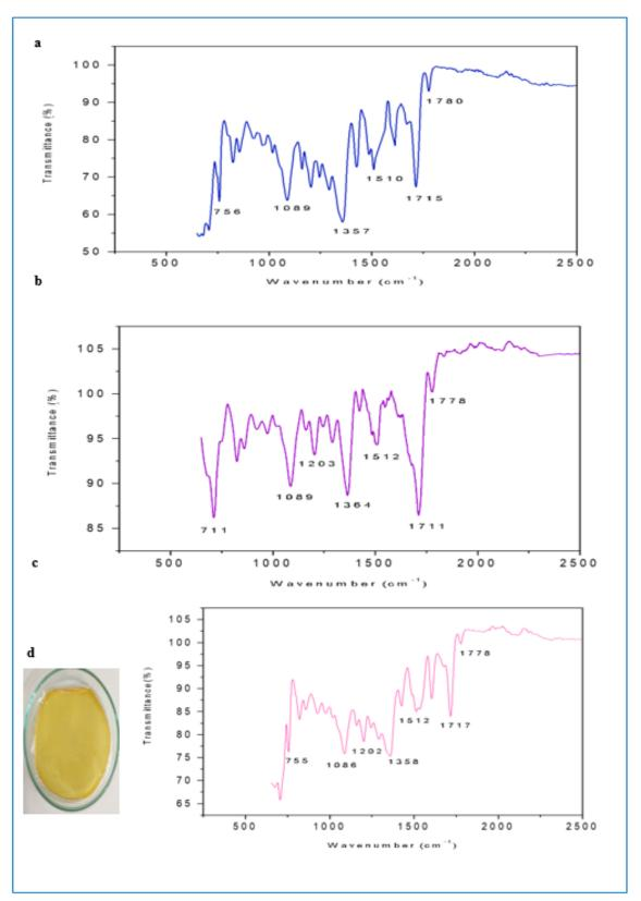
Fig. 4: FTIR spectra of 10  $\mathbf{a}$ , 20  $\mathbf{b}$  30 wt. %  $\mathbf{c}$  (Pr(BTC)(H<sub>2</sub>O)<sub>6</sub>)-Matrimid® MMMs and screenshot  $\mathbf{d}$  of 30 wt.% MMM.
